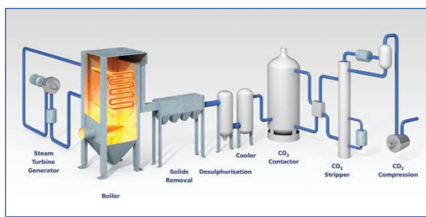
Figure 2. Post combustion capture coal fired power plant.
